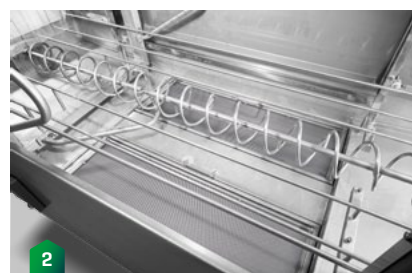
1 DLWA 180 Ecoline 2 Box transport by means of stainless steel spiral
